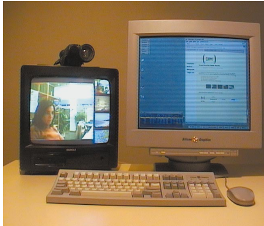
Figure 1. Typical configuration for an analog media space node.
